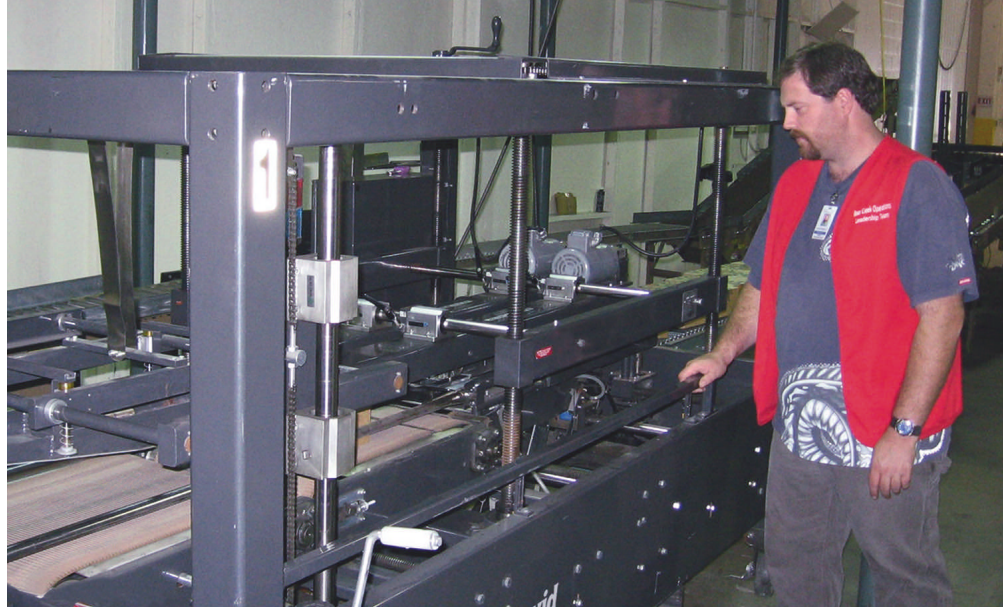
Line supervisor Ernie Pritchett looks at one of the mobile tape-sealing machines that can be transported and operated outdoors.
