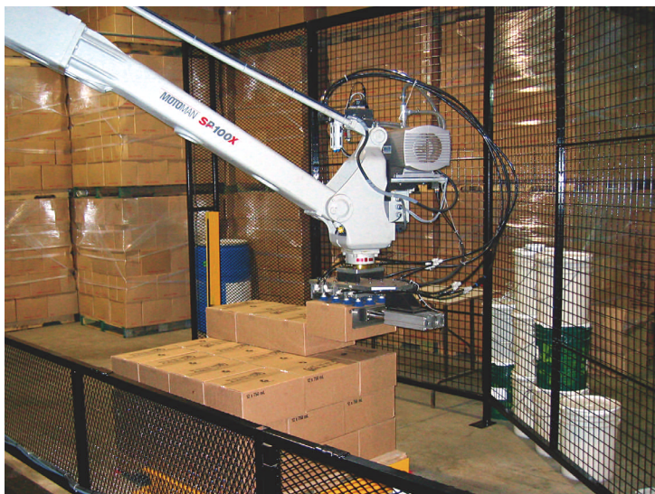
Cases of product enter the robot cell via a single-lane, powered infeed conveyor. Sensors on the conveyor indicate that the cases are in the proper location and are ready for robotic pickup.
