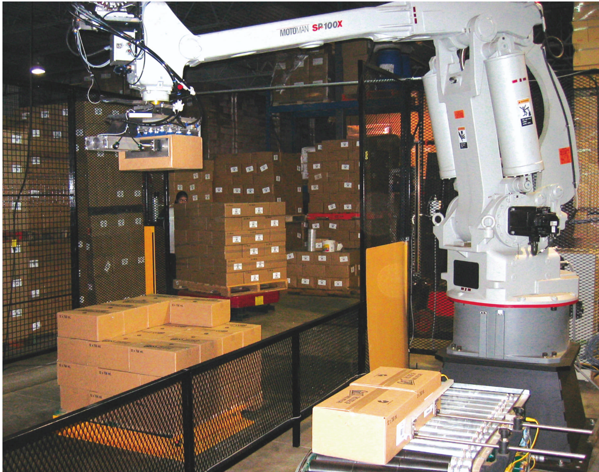
The palletizing robot is equipped with a custom-designed, multifunction gripper that uses a single-zone vacuum device along with a pneumatically actuated mechanical side plate to securely grab and transfer the cases, regardless of their size or weight.
