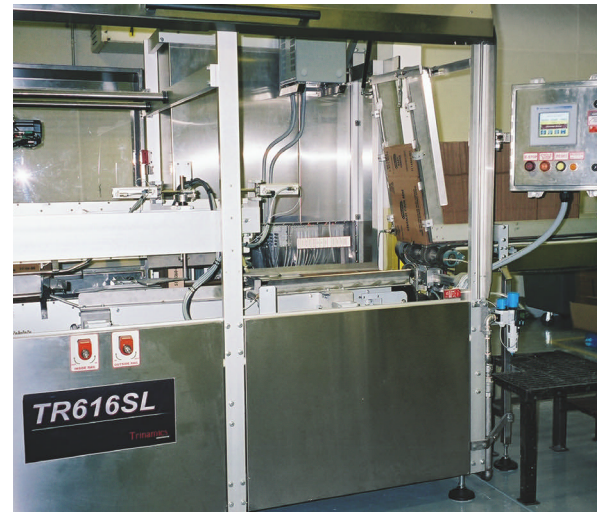
The case packer has been designed and engineered for rapid changeover. Many parameters are servo driven, and their presets are recalled through the human/machine interface.
