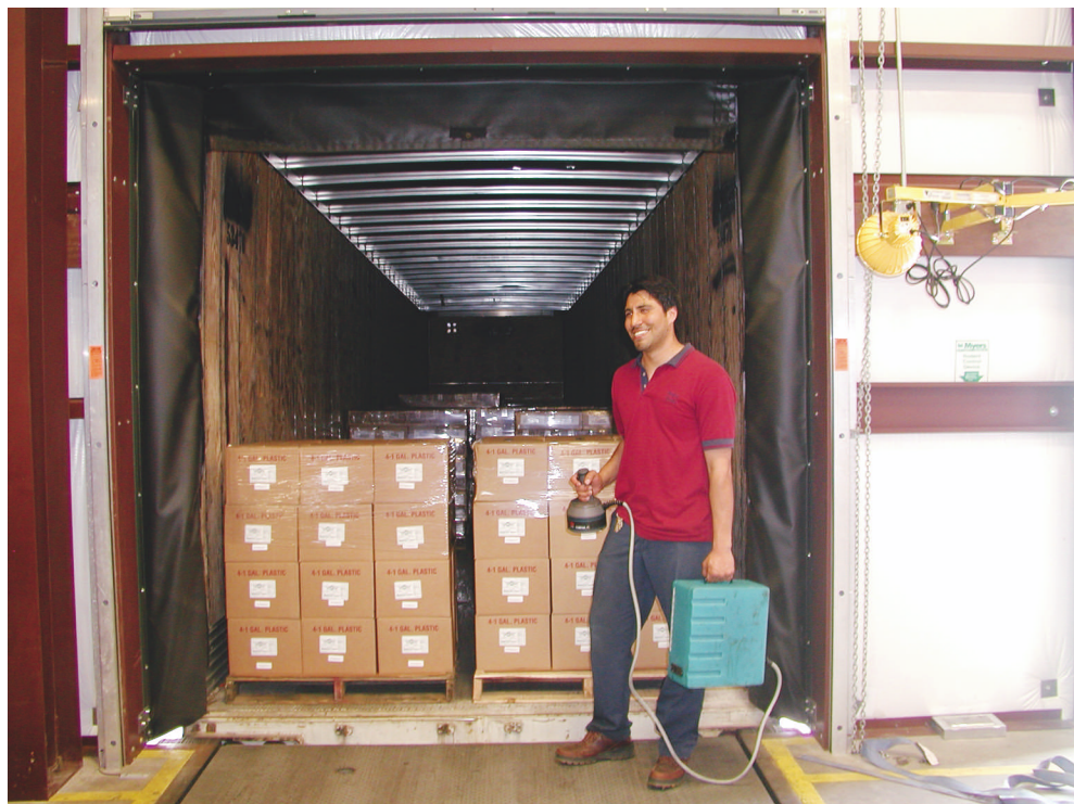
An operator holds one of Renfro Foods' compact tabletop induction-cap sealers, which it uses to seal whole trailer loads of salsas, sauces and other foods.
