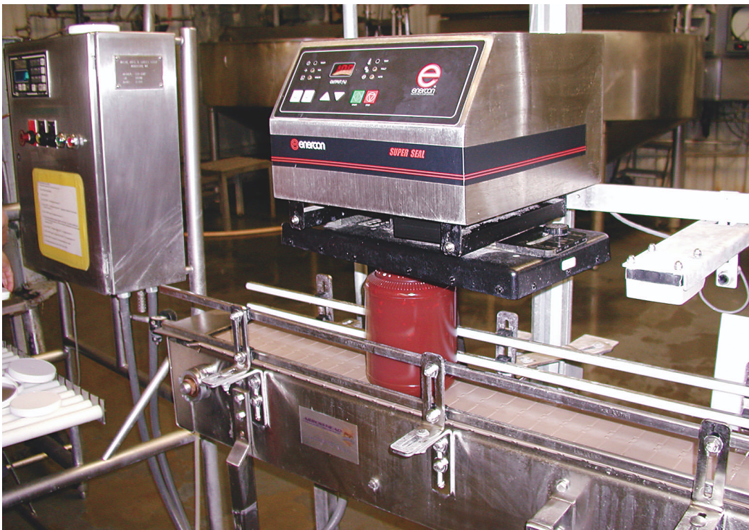
The in-line, fully-automatic induction sealer, above, allows Renfro Foods to anticipate additional growth expectations for years to come. It seals larger, foodservice jars and jugs in sizes from 1 to 5 gal.
